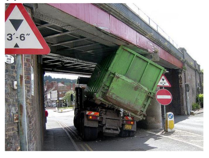
excites a dynamic response in the passing vehicle, potentially enabling detection of the damage through analysis of the vehicle response. As part of this project I have developed a method for the detection of bridge damage through comparison of apparent profiles sensed by the passing vehicle. The apparent profile is a virtual longitudinal profile which, when applied to a vehicle, invokes the same measured response to the crossing of a bridge.
