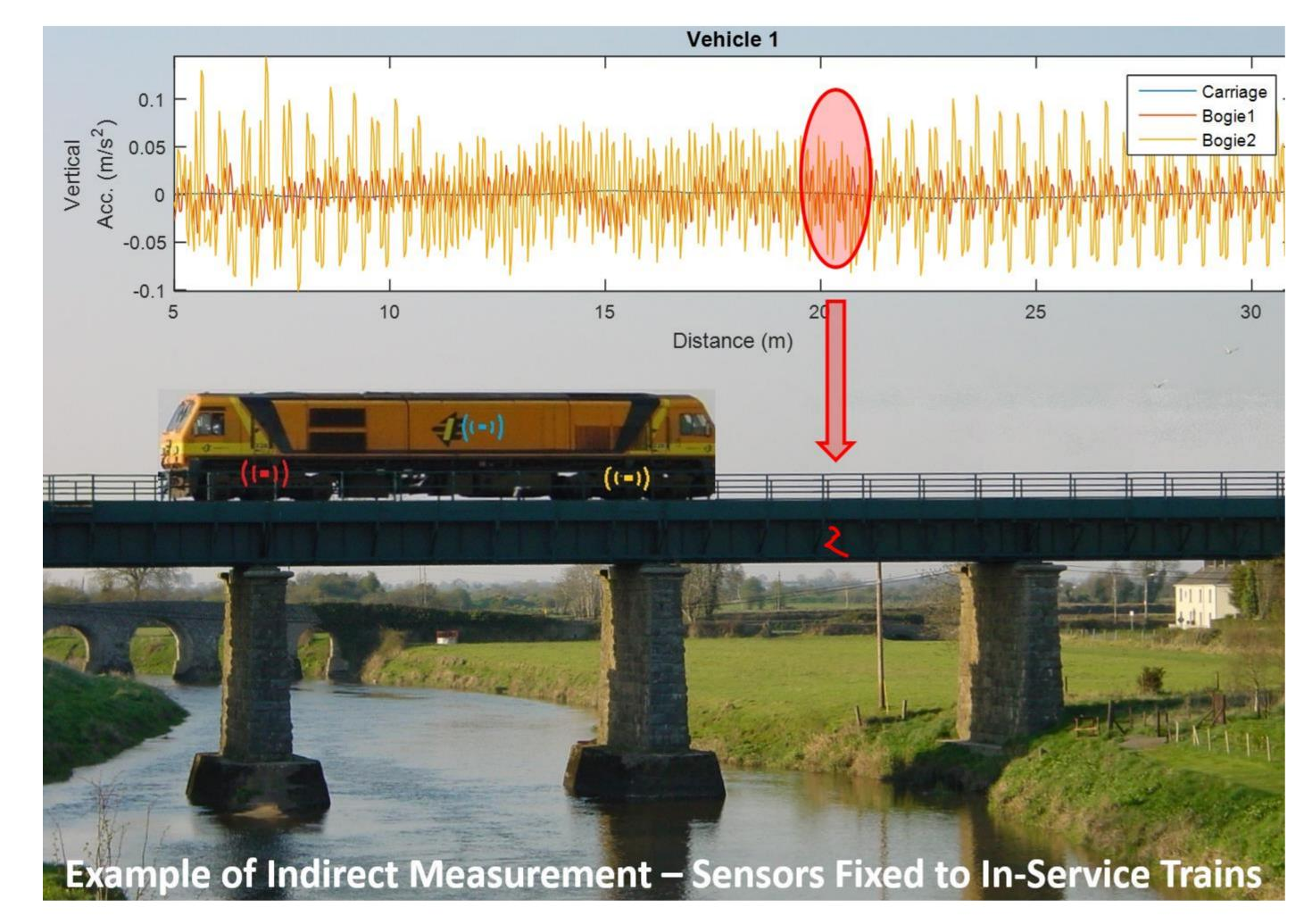
**Bridge Damage Detection through Apparent Profile**
