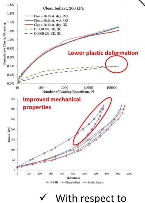
Use of Pneumatic Unbound Material Analyser (PUMA) test to analyse in small scale the influence of bitumen emulsion on ballast mechanical behaviour PUMA TEST
