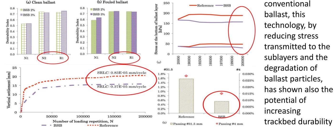
✓ Full-scale box tests highlighted the potential for BSB to reduce ballast problems associated with its unbound nature such as settlement and particle deterioration, limiting therefore the need for maintenance and increasing trackbed durability
