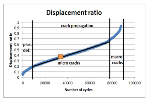
Micro cracking predominates at 50% stiffness reduction. Macro cracks appear around 70% stiffness reduction. Failure criteria differs from HMA and should be stablished.
